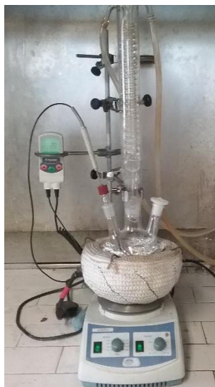
Figure 12 – Experimental set-up of the acetylation reaction.
